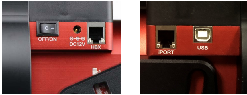
Figure 24. Ports for cables
