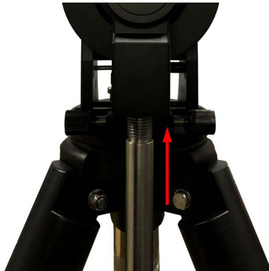
Figure 18. Install CW shaft
