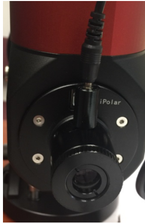
Figure 26. Connect polar scope LED
