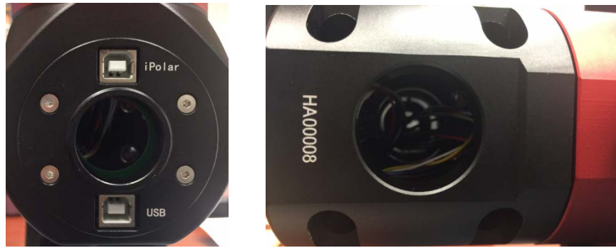
Figure 6. Openings for custom cable management
