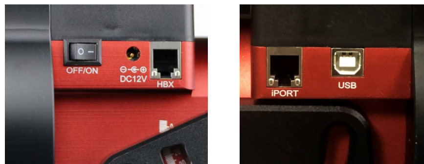
Figure 2. Ports on a CEM40 mount
