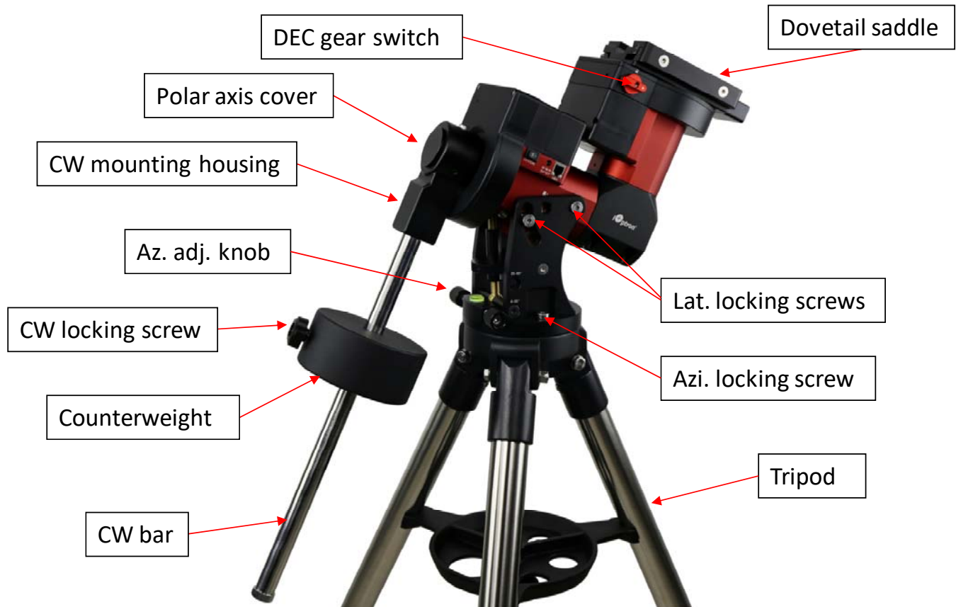
Figure 1.CEM40 mount assembly
