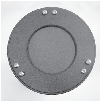
Figure 11. The back end of the optical tube (bottom of the primary mirror cell). The three pairs of collimation screws adjust the tilt of the primary mirror.
