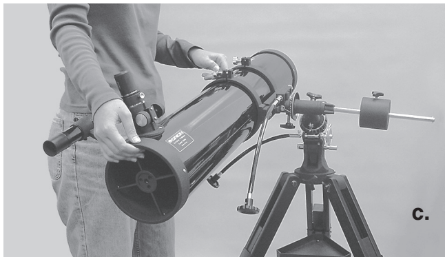
Figure 4a, 4b, 4c, 4d. Proper operation of the equatorial mount requires that the telescope tube be balanced on both the R.A. and Dec. axes. (a) With the R.A. lock knob released, slide the counterweight along the counterweight shaft until it just counterbalances the tube. (b) When you let go with both hands, the tube should not drift up or down. (c) With the Dec. lock knob released, loosen the tube ring lock clamps a few turns and slide the telescope forward or back in the tube rings. (d) When the tube is balanced about the Dec. axis, it will not move when you let go.
