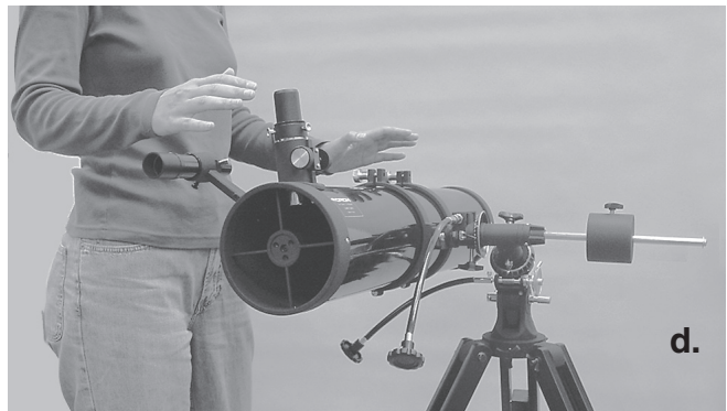
Figure 4a, 4b, 4c, 4d. Proper operation of the equatorial mount requires that the telescope tube be balanced on both the R.A. and Dec. axes. (a) With the R.A. lock knob released, slide the counterweight along the counterweight shaft until it just counterbalances the tube. (b) When you let go with both hands, the tube should not drift up or down. (c) With the Dec. lock knob released, loosen the tube ring lock clamps a few turns and slide the telescope forward or back in the tube rings. (d) When the tube is balanced about the Dec. axis, it will not move when you let go.
