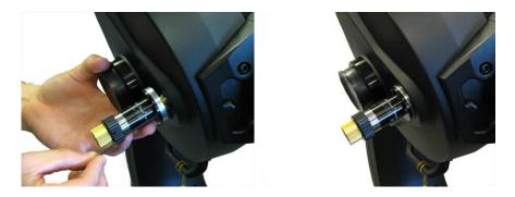
Use the three included screws to attach the SCT MicroFocuser to the telescope. You are now ready to head out under the stars! Use the black knob for coarse focus and the brass knob for fine focus (10:1 ratio). Note that the telescope will likely be pretty far out of focus, so you may need to turn the focus knob quite a few times to reach focus.
