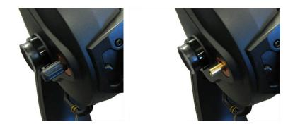
Begin by removing the black rubber focus knob from the scope. This knob simply pulls off the brass focus cylinder.
