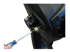
Thread the screw back into the end of the focus shaft.
