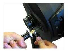
Thread the MicroFocuser into the brass stop. Hold the stop with a wrench and the black focus knob with the other hand to tighten the stop. *This stop MUST be tight to secure the MicroFocuser to the focus shaft.*
