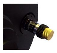
When there is only about 1/4" left to go, simply push the focuser the rest of the way in. This will take up some of the change in focus from when you removed the original focuser, making it quicker to return to focus the first time you use your telescope after the SCT MicroFocuser installation.
