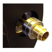
Turn the brass focus shaft counterclockwise to remove it from the threaded focus rod. This will take quite a few turns. Once the bearing assembly is removed, only the threaded focus rod (which pushes and pulls on the mirror cell to focus the telescope) will be left sticking out of the telescope as below.
