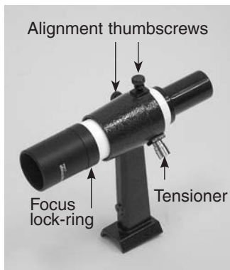
Figure 2a. The 6x30 finder scope and bracket
