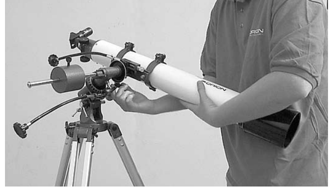
Figure 3c. Preparing the telescope to be balanced on the Dec. axis by first releasing the Dec. lock knob.
