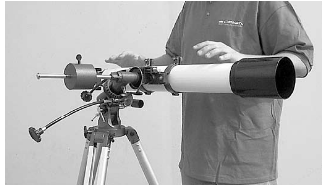
Figure 3e. Telescope is now balanced on the Dec. axis, i.e., it remains horizontal when hands are released.
