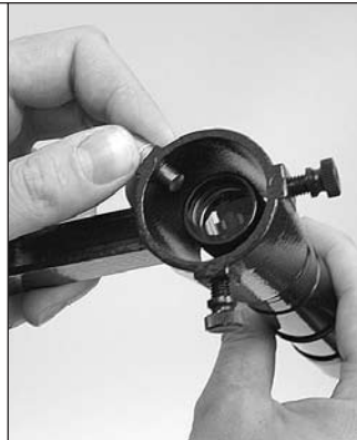
Figure 3b. Inserting the finder scope into the finder scope bracket
