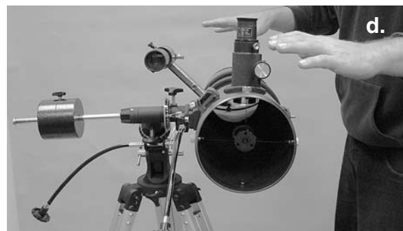
Figure 4. Proper operation of the equatorial mount requires that the telescope tube be balanced on both the R.A. and Dec. axes. (a) With the R.A. lock knob released, slide the counterweight along the counterweight shaft until it just counterbalances the tube. (b) When you let go with both hands, the tube should not drift up or down. (c) With the Dec. lock knob released, loosen the tube ring lock clamps a few turns and slide the telescope forward or back in the tube rings. (d) When the tube is balanced about the Dec. axis, it will not move when you let go.
