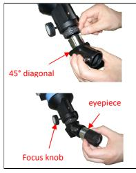
**Insert 45º diagonal:** Insert the diagonal into the eyepiece side of the telescope. Tighten the thumbscrews to a firm feel only.
