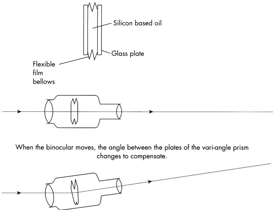
**Fig. 2.16** Image stabilization with Canon's vari-angle prism
