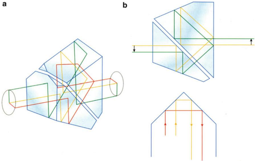
**Fig. 2.11** Image reversal in Pechan roof prism
