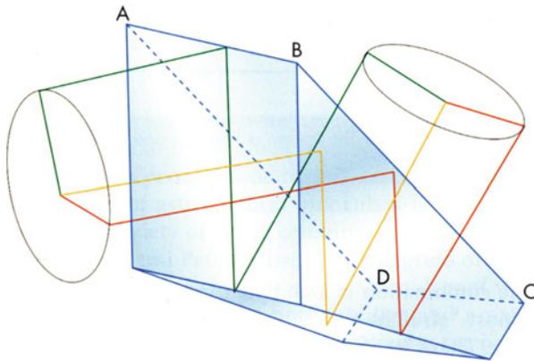
**Fig. 2.12** Semi-pentaprism (45° deviation prism)
