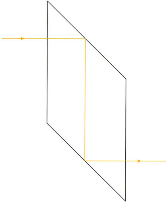
**Fig. 2.14** Rhomboid prism. This prism displaces the axis
