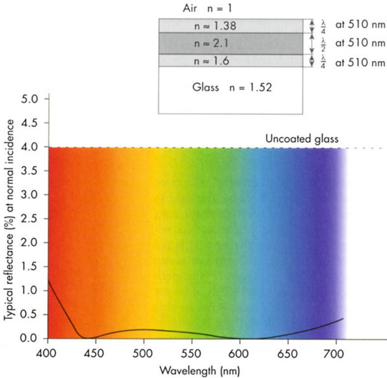
**Fig. 2.20** Broadband multi-coated optics: triple layer coating
