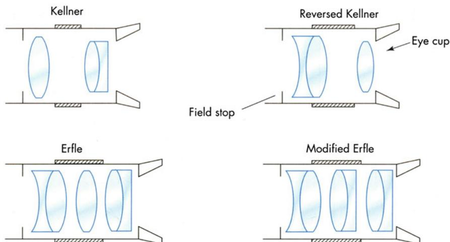
**Fig. 2.2** Some common binocular eyepieces
