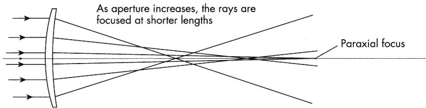
**Fig. 2.24** Spherical aberration in a converging lens
