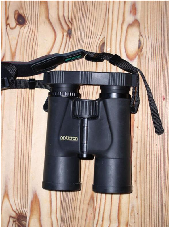
**Fig. 2.31** Roof-prism center focus
