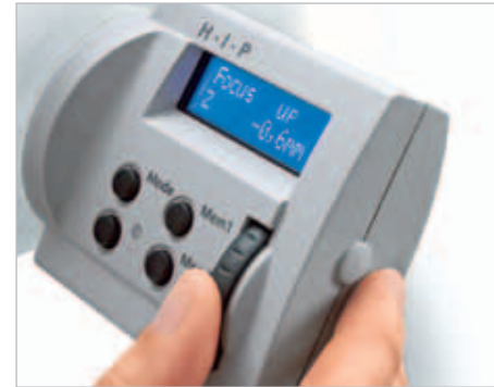
The Focus Motor moves slowly when the wheel travels small distances and faster when it travels greater distances.
