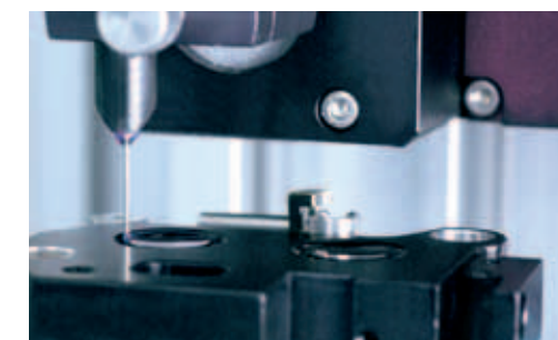
Once the lens has been pushed into position, it is fixed in place immediately. A 0.5 mm thick cannula is used by high-precision tools to automatically apply continuous adhesive beads with high accuracy and precision.
