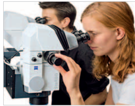
Position and rotate the LED pointer to mark interesting spots on your specimen.
