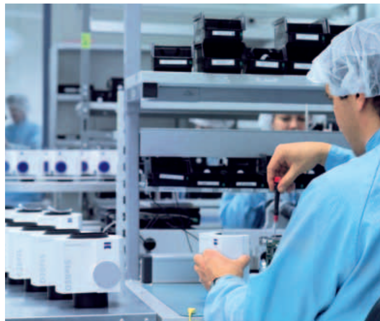
Fast, flexible, effective: SteREO Discovery stereo microscopes undergoing final assembly at the Carl Zeiss Microscopy GmbH clean rooms in Jena. The method? One-piece continuous flow manufacturing based on value stream design criteria.
