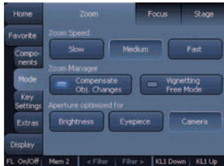
The Axio Zoom.V16's eZoom is coupled with a motorized iris: simply press the button for the zoom mode you need.
