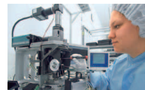
The precise movement of all the moving optical elements in the optical train is programmed on the zoom lens system adjustment device. Around 7,000 support points are analyzed in a computer for this purpose. This ensures that each individual stereo microscope gets its own fine-tuning calibration and its own individual zoom curve.
