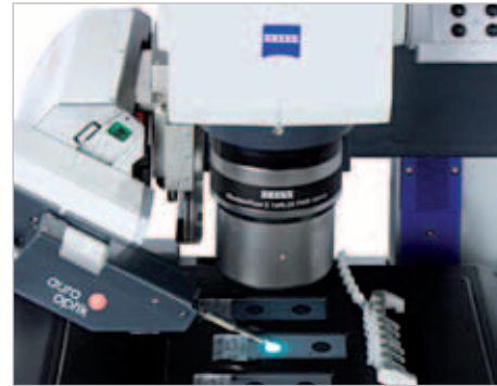
The 6X stage top holder and the 6X 237 x 157 mm slide tube insert can be used to isolate sperm from a mixture of cells and transfer them to tubes.
