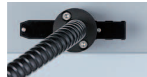
Position 3: ■ EpiRel slider at "relief contrast" end position (right) ■ This end position is available in both directions ■ Direction of illumination tilted 1°
