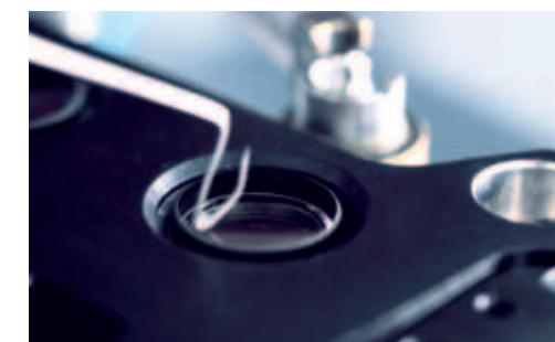
... a moving micro clapper on the computer-controlled glue levelling robot performs the necessary fine adjustments independently.
