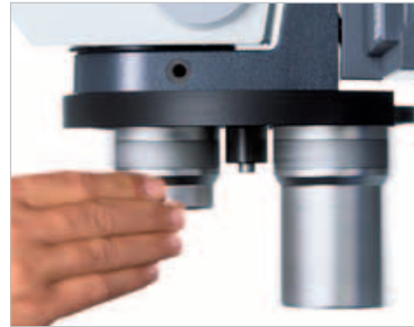
The Objective nosepiece Z, 2x cod you to change objectives quickly and conveniently. Thanks to the turret's position-encoding feature, you can use SYCOP 3 to automatically read optical parameters such as magnification, field of view diameter, resolution, and depth of field. In addition, you can focus non-parfocal objectives automatically with the Focus Motor after activating the Parfocality Manager feature.
