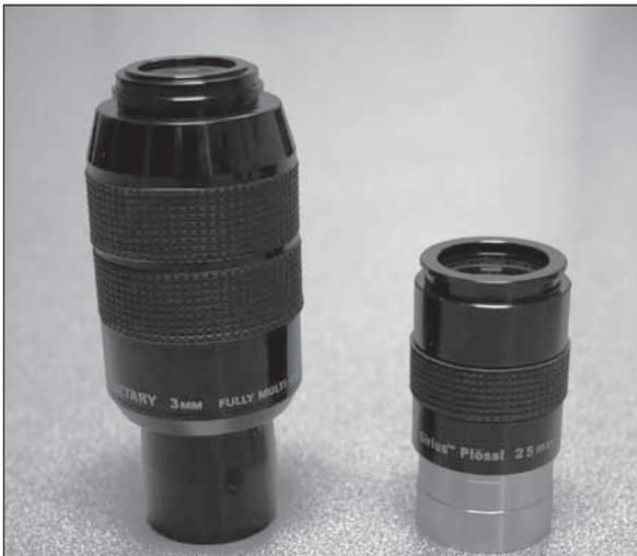
**Figure 2.** Examples of two eyepieces with housing diameters that are compatible with the SteadyPix EZ. The 25mm Sirius Plossl (right) has a housing diameter of 35mm; the 3mm Edge-On Planetary eyepiece has a housing diameter of 45.5mm. Both eyepieces are shown with their rubber eyecups removed.
