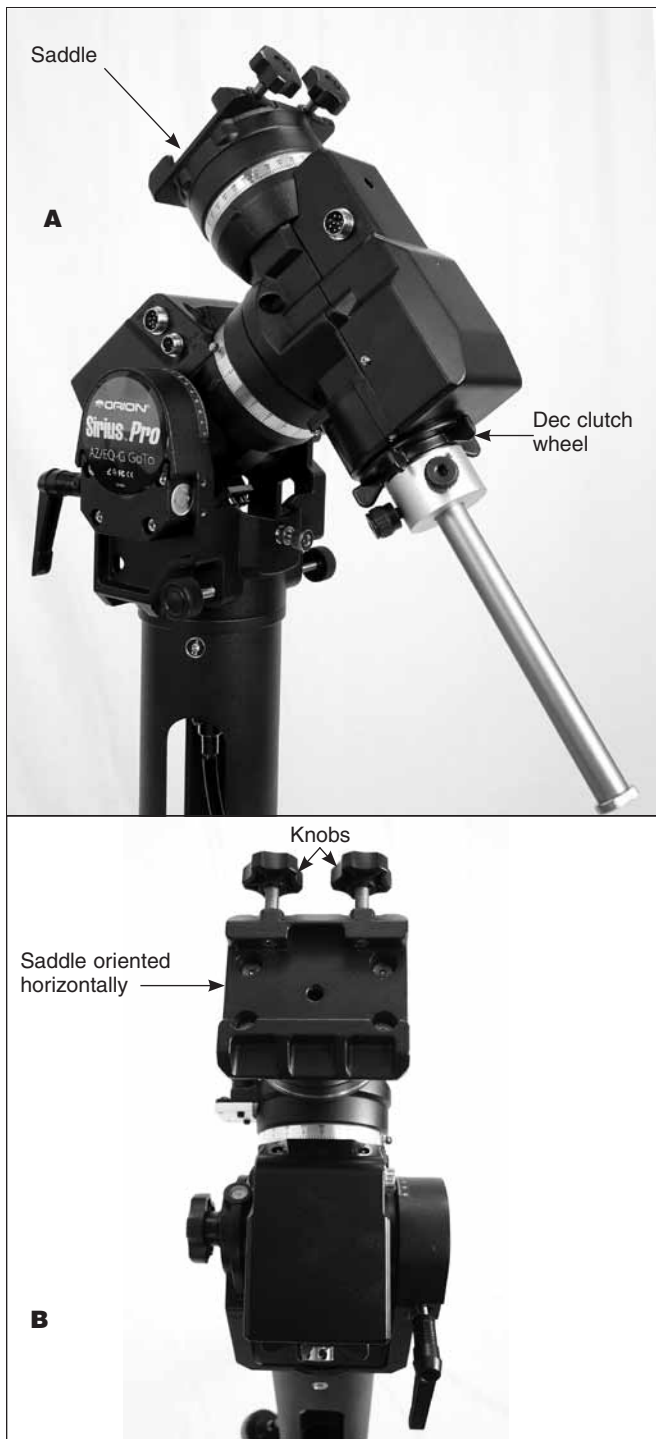
Figure 12. A) Loosening the Dec. clutch wheel lets you rotate the dovetail saddle to a horizontal position. Be sure to tighten the clutch before installing your telescope! B) Tighten the two rosette knobs to secure your telescope in place.
