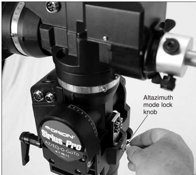
Figure 16. The altazimuth mode lock knob secures the mount in position for use in altazimuth mode.
