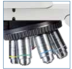
Revolving sextuple reversed nosepiece on ball-bearings
