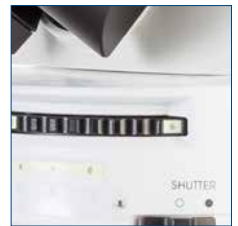
For slider with 1λ retardation plate for observation of monosodium crystal deposition (gout) and for DIC slot (DIC ready)
