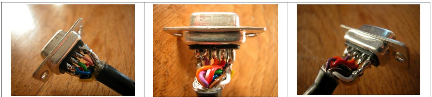
If you open the cable, make sure you put the cover back and water proof. Use the right fixing ring for this.
