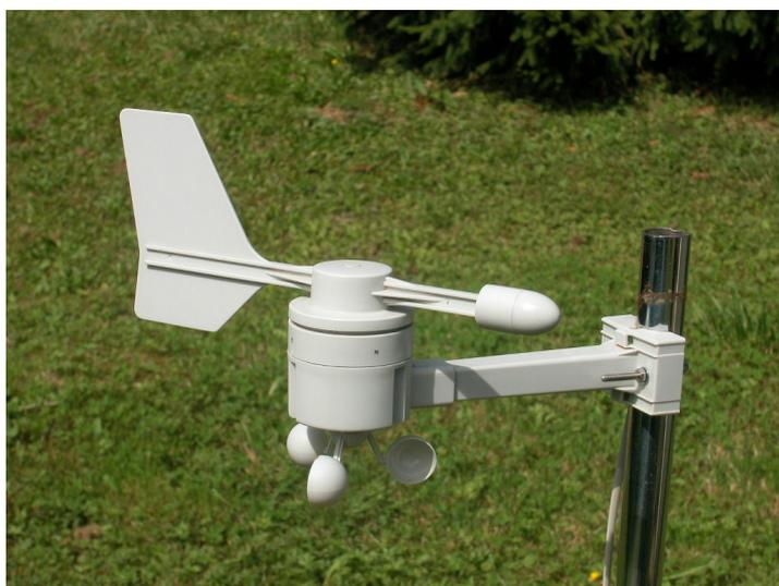
***Wind sensor installed on a pole***
