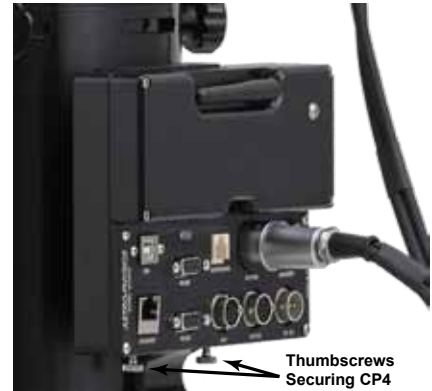
Mach1GTO with CP4 Attached to Pier
