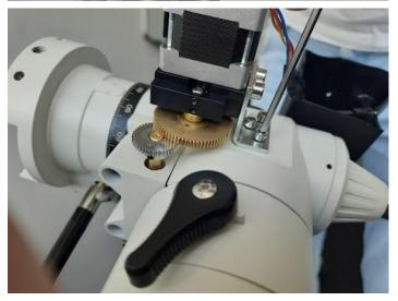
5.) Place the plastic cover over the motor, and attach it with the small black screws.
