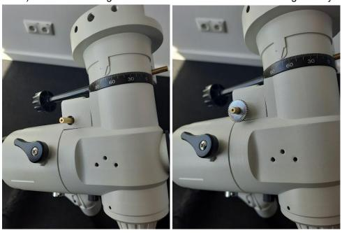
2.) Attach the RA-Motor on the 3 small holes near the RA worm axis. Don't tighten the screws yet.
