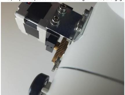
4.) Tighten the 3 screws of the RA Motor and the set screws at the small gear.
