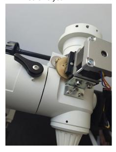
3.) Adjust the position of the motor and gear wheel, to engage the gears with each other.
