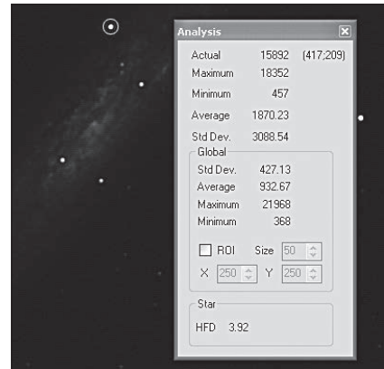
Figure 10. The Analysis window displays useful data about your image. Hovering the mouse over a star will also display the HFD value which indicates the star diameter for best focus.
