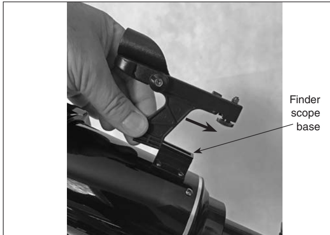
Figure 11. Slide the red dot finder scope's bracket into its base.
