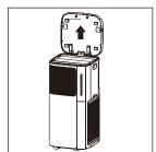
9 Take out the two filters and remove their package and then put them back into the machine.
