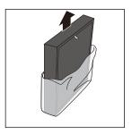
4 Put the unpacked air purification filters back into the appliance.
